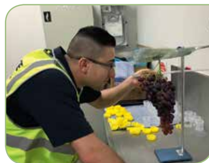
Produce Quality Inspector, Behrang Saber, measuring a bunch of Crimson Seedless grapes at the Rudge Produce Laboratory in Melbourne. Each individual berry was measured for Brix, acid, size and its 3D position in the bunch.
