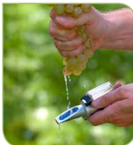
Measuring brix is vital to ensure grapes are mature and ready to eat.
